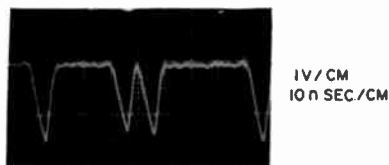
Fig. 18—Output waveform at 90^{\circ}\text{C} .
